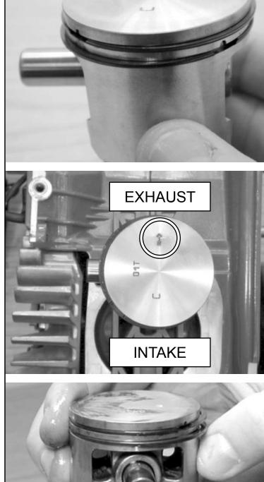
13.18 Align piston in correct orientation.
